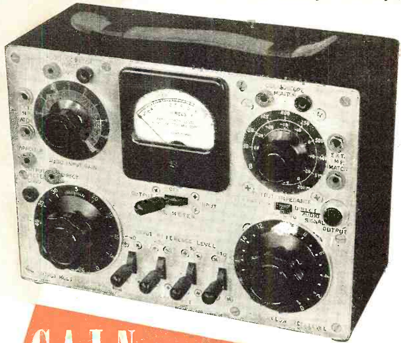
Fig. 1. Front view of gain measuring set.
